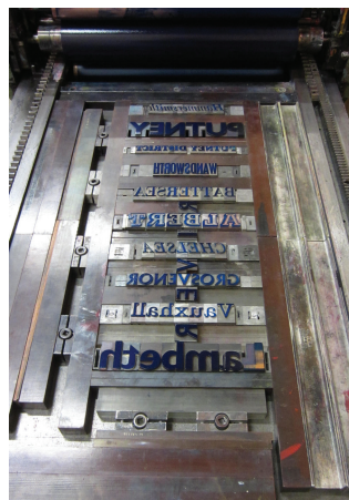
Figure 1.2: Printing Press letters configuration—arranged backwards
